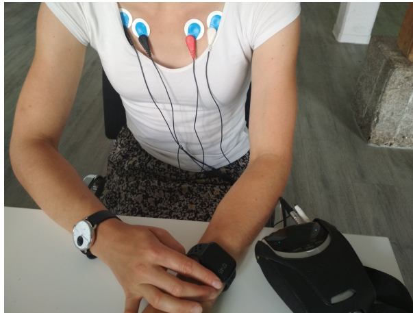
Figure 4.1: ECG recording setup. A participant wearing the Apple Watch (left wrist) and Withings Scanwatch (right wrist). The electrodes of the reference ECG are connected just below the collarbone.
