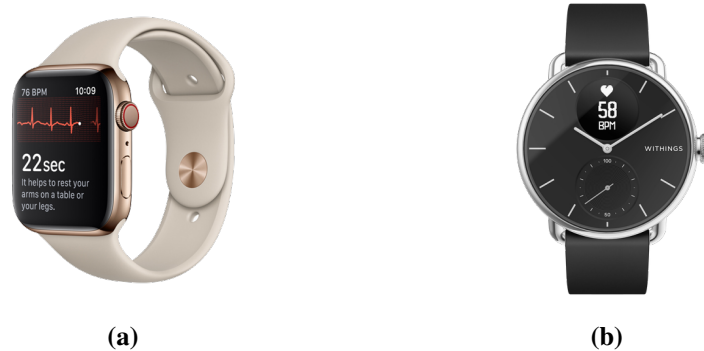
Figure 2.3: Smartwatch with ECG functions. (a) Apple Watch Series 4 [App18] (b) Withings Scanwatch [Wit22a]
