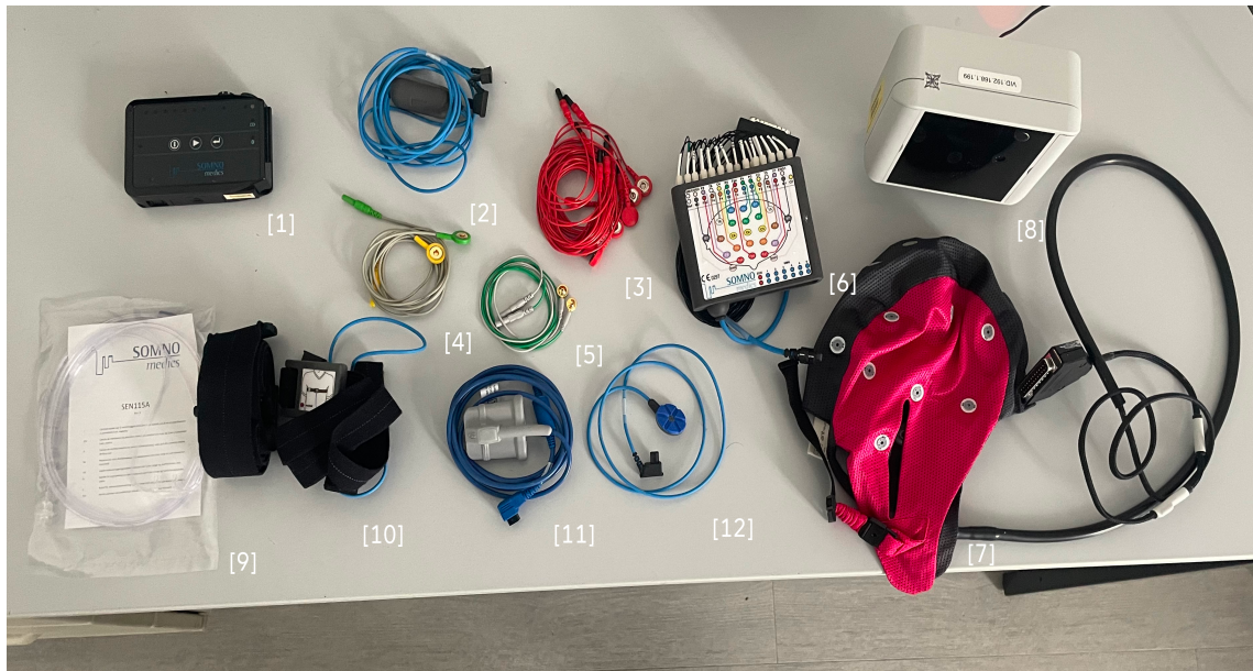
Figure 5.1: An overview of the different components of the utilised SOMNO HD eco PSG system: [1] somno hub, [2] leg EMG electrodes, [3] arm and chin EMG electrodes, [4] ECG electrodes, [5] EOG electrodes, [6] Hub for EEG and EOG, [7] EEG electrode cap, [8] night camera, [9] nose tubes, [10] abdomen and torso straps, [11] finger pin, [12] microphone
