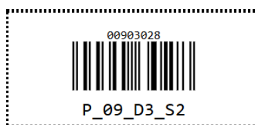
Figure 3.6: Generated barcode. The digits above the code are the barcode value. The label below the barcode provides information about the participant and the sample to which the barcode belongs.
