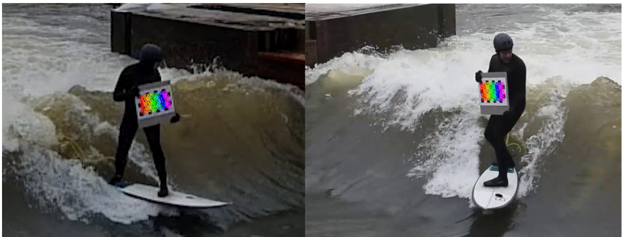
Figure 3.5: Checkerboard corners detection from the back-left and back-right camera views
