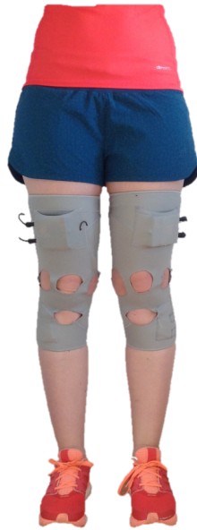
Figure 5.1: The two sensor equipped sleeves which were used for the data acquisition. Holes have been cut in the sleeves to mark the positions, where the passive markers of the motion capturing system are placed.
